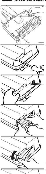
Remove the replacement belt from the storage channel.
